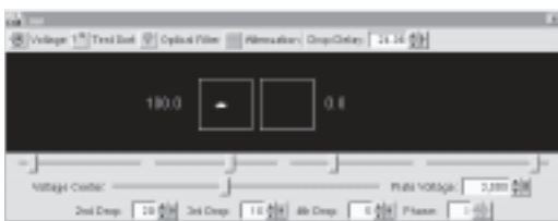
Figure 77 Optimized Drop Delay Profile with Spherotech Drop Delay Calibration Particles.
